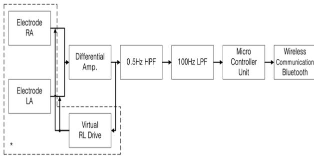
**Fig. 1** Block diagram of the electrocardiogram measurement. Virtual RL Drive give a feedback to electrode RA and LA, so 2-Electrode ECG Module can minimize the effect of motion artifacts during exercise(\*).
