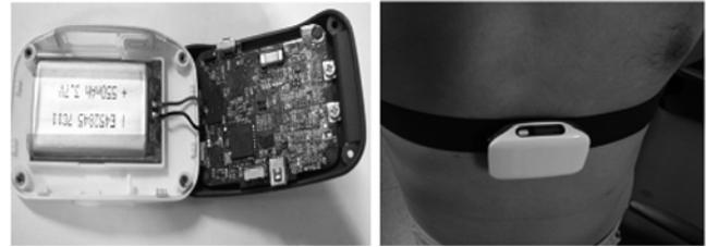
**Fig. 1.** Wearable ECG system and sensor placement.
