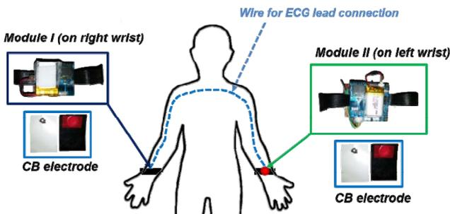
Fig. 1. “NohChon” Wrist ECG Wearable Device
