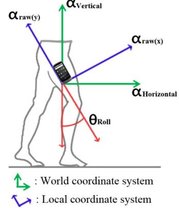
Figure 1. Accelerometer coordinate system in WCS and LCS
