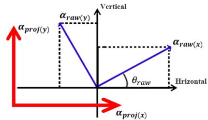
Figure 2. 2D-projection from LCS into WCS
