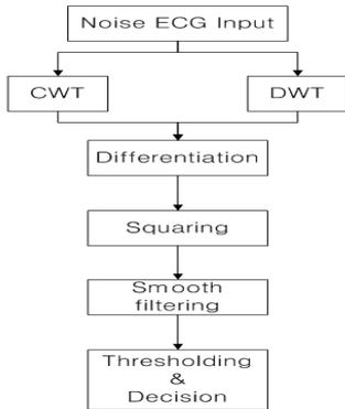
Figure 3. QRS Complex detection flowchart
