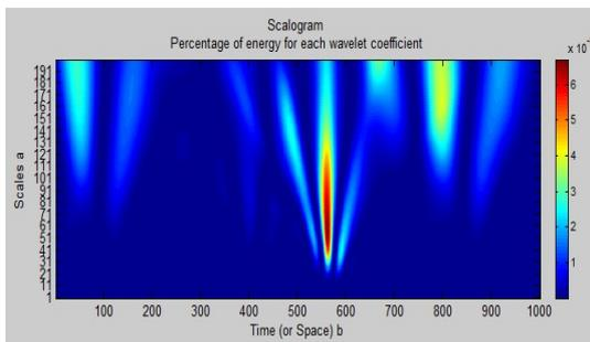
Figure 1. Scalogram shows Wavelet on a Scale  $a=1\sim 200$  per beat that was traced by Coefficient Daubechies3 function
