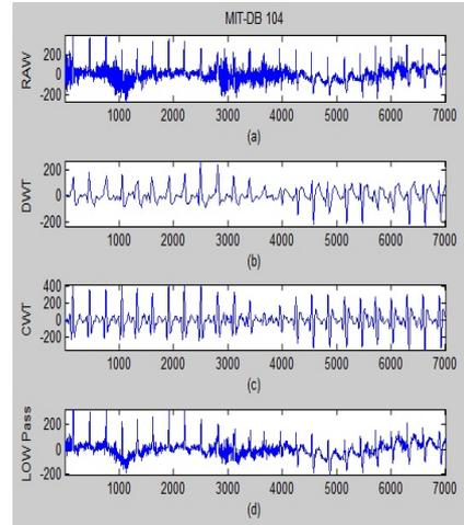
Figure 4. (a) MIT-DB 104, (b) Data after DWT (c) Data after CWT (d) Low-pass filter with  $f_c=25\text{Hz}$
