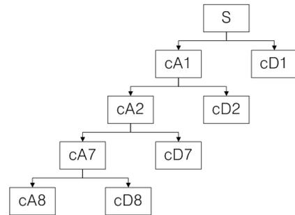
Figure 2. Diagram of ECG with 8 Level Decomposition
