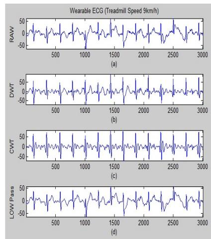
Figure 5. (a) Speed of 9km/h on the treadmill (b) Data after DWT (c) Data after CWT (d) Low-pass filter with  $f_c=25\text{Hz}$
