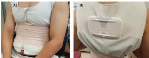
Figure 1. Subject wearing the Heart Cycle vest. A) Front side of the vest and elastic strap; B) Back side of the vest showing the measuring device.
