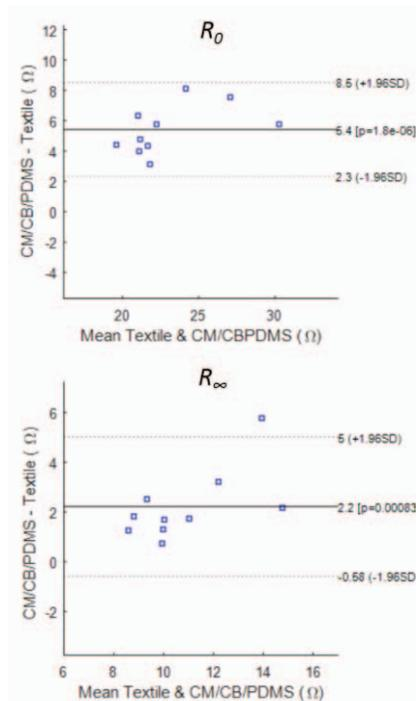
Figure 4. Bland-Altman plots for  $R_0$  and  $R_\infty$  values between CM/CB/PDMS and textile electrodes.
