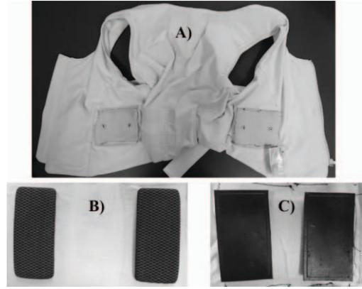
Figure 2. A) Heart Cycle vest with snap connectors; B) Original embedded textile electrodes; C) Carbon black PDMS electrodes attached to the vest with two electrodes on both sides
