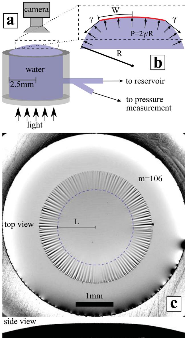
**Fig. 1.** (a) Experimental set-up. (b) Schematic side view of the drop and sheet. The sheet has radius  $W$  and the exposed part of the drop beneath has radius of curvature  $R$ . (c) Top and side views of the wrinkled sheet on the drop. The radius of the unwrinkled region ( $L$ ) and the wrinkle angle ( $\frac{2\pi}{m}$ ) are computed by analyzing the top image (SI.7).
