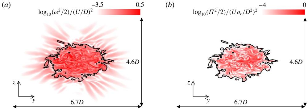
FIGURE 2. Vertical cross-sections of (a) enstrophy and (b) potential enstrophy fields at  $Nt=21$  for Case 1. The solid black line shows the wake edge.
