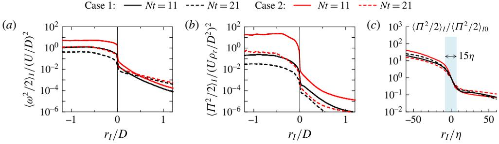
FIGURE 3. Conditional mean profiles of (a) enstrophy  $\omega^2/2$  and (b) potential enstrophy  $\Pi^2/2$ . (c) Conditional mean potential enstrophy  $\Pi^2/2$  against the distance from the wake edge normalized by the Kolmogorov length scale  $\eta$ . In (c), the conditional mean potential enstrophy is normalized by the value at the wake edge  $\langle \Pi^2/2 \rangle_{I0}$  at  $r_I = 0$ .
