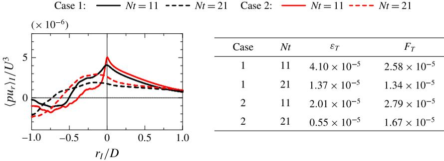
FIGURE 4. Conditional averaged profiles of the radial energy flux  $pu_r$ . The line types are the same as in figure 3. The table shows values of the total kinetic energy dissipation rate  $\epsilon_T$  and the total energy flux  $F_T$  normalized by  $U_0$  and  $D$ .
