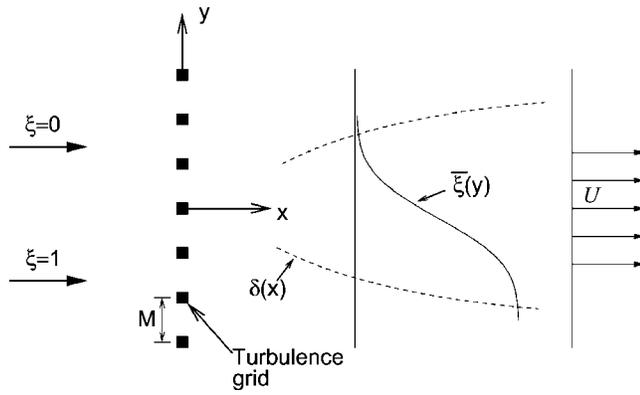
FIG. 1. Schematic of a scalar mixing layer.
