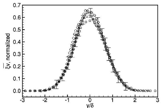
FIG. 13. Profiles of the scalar flux normalized by  $I_{max}$  and  $v_{rms}$ . Symbols are the same as in Fig. 10. The line and error bars represent the data from Ref. 8.
