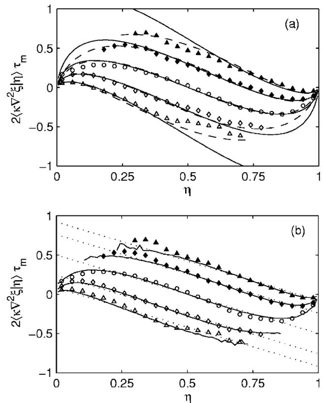
FIG. 9. The conditional scalar diffusion rate normalized by the mixing time scale,  $\tau_m = \xi^2 / \bar{\chi}$ , at various cross-stream locations. Symbols are the same as in Fig. 4. In (a), Mortensen's model is shown for both the full model (solid line) and the homogeneous part (dashed line) using the  $\beta$ -PDF. In (b), Sawford's Lagrangian simulation (solid lines) and the IEM model (dotted lines) are shown.
