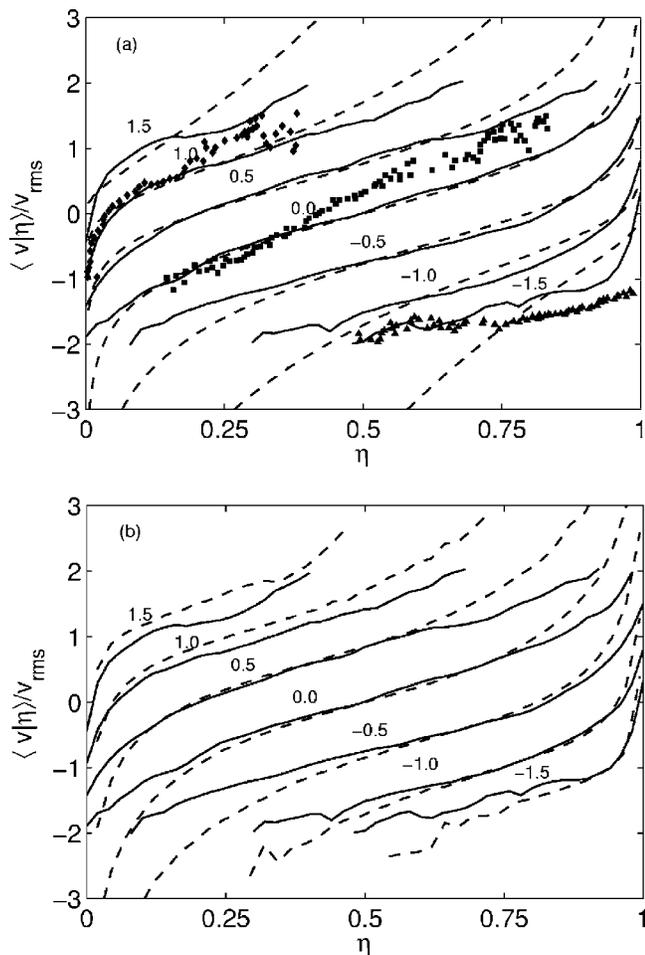
FIG. 3. The conditional mean transverse velocity at various cross-stream locations. The solid lines denote the DNS results with the numbers above each set of data indicating the  $y/\delta$  value. The symbols in (a) are from Ref. 3 for  $x/M=19$  and  $y/\delta=-1.3, 0.1,$  and  $1.28$ . The dashed lines in (a) correspond to (6) computed with the presumed  $\beta$ -PDF for the same positions as the DNS. The dashed lines in (b) correspond to the Lagrangian simulation.
