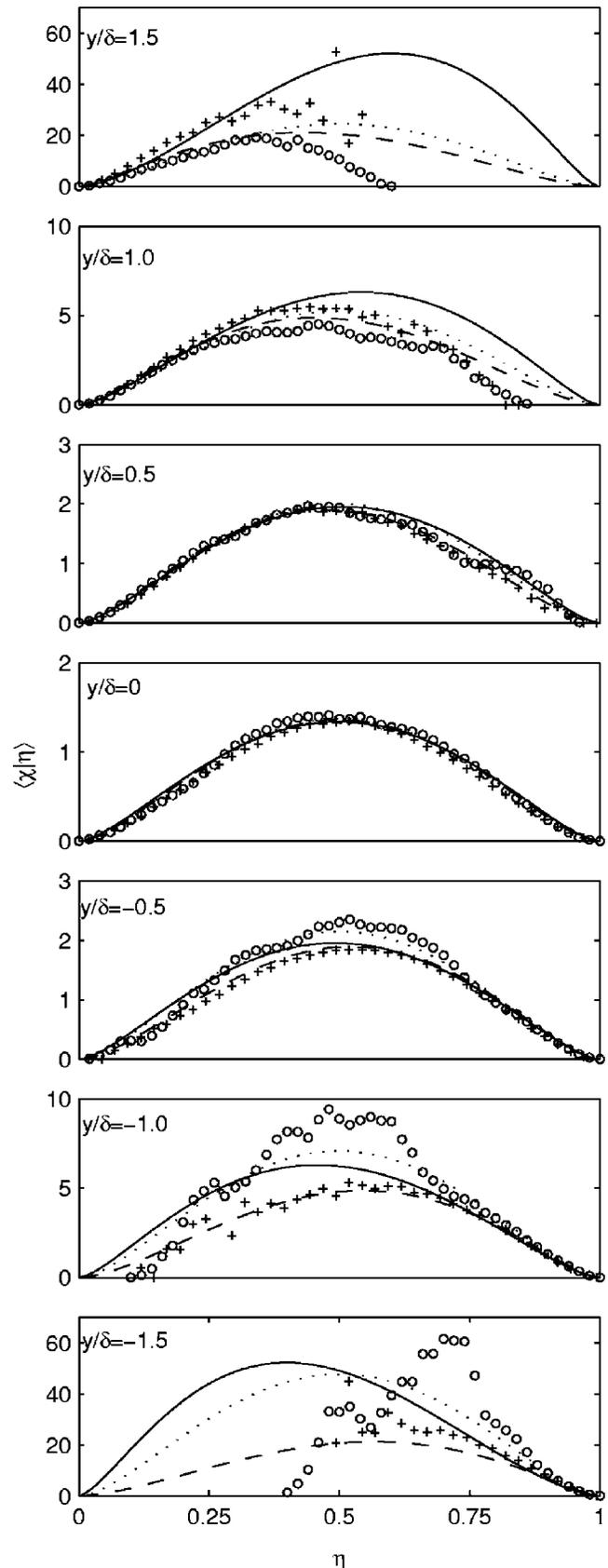
FIG. 6. The conditional scalar dissipation rate at various cross-stream locations normalized by  $\bar{\chi}$ . Different transverse locations are shown in each panel. Equation (12) is calculated from the  $\beta$ -PDF and Mortensen's full model is represented with solid lines, whereas the homogeneous part is represented with dashed lines. The counterflow model is represented with dotted lines and the Lagrangian simulation results are represented with "+". Open circles are the DNS data.
