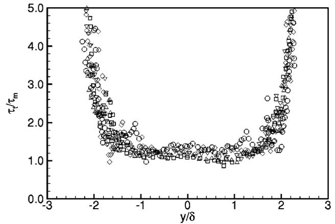
FIG. 16. Ratio of the turbulent time scale to the mixing time scale. Symbols are the same as in Fig. 10.
