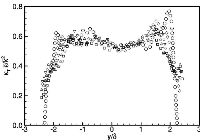
FIG. 15. Profiles of the normalized turbulent diffusivity,  $\kappa_T u_{rms} \delta$ . Symbols are the same as in Fig. 10.
