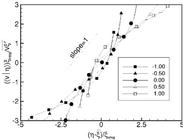
FIG. 5. The conditional mean transverse velocity at various cross-stream locations. The data have been normalized in accordance with the linear model.
