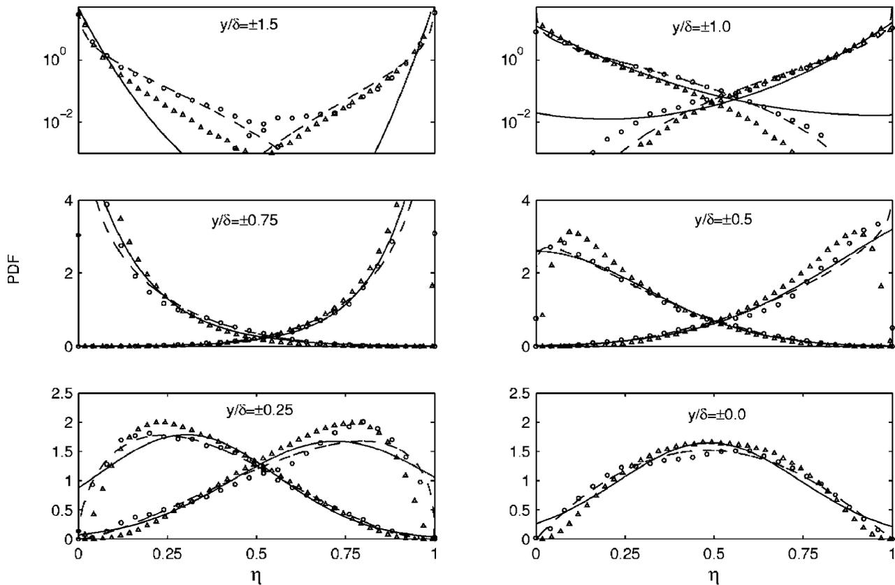
FIG. 2. Probability density of  $\xi$  at different transverse locations. DNS is represented with an  $\circ$ , the  $\beta$ -PDF with a dashed line, the SML-PDF with a solid line and the Lagrangian simulation with a triangle. Note that the curves for high  $y/\delta$  values are plotted on a log scale.
