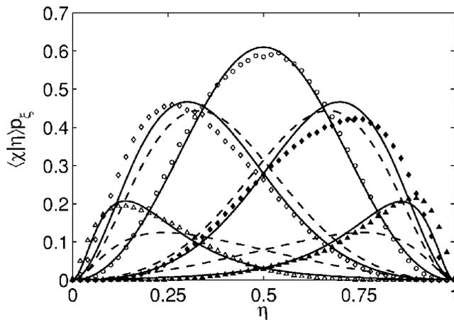
FIG. 8. The conditional scalar dissipation rate times the PDF at various cross-stream locations. The PDF is presumed with the SML-PDF. Symbols are the same as in Fig. 4. The solid line represents Mortensen's full model, whereas the dashed line is the homogeneous part.
