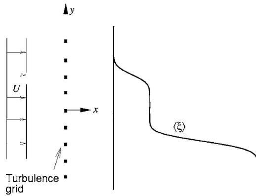
FIG. 1. Schematic of the double scalar mixing layer.
