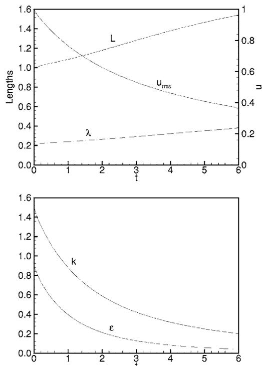
FIG. 3. The velocity integral length scale, Taylor microscale, and rms velocity versus scaled time (top); below, the turbulent kinetic energy and its dissipation rate.
