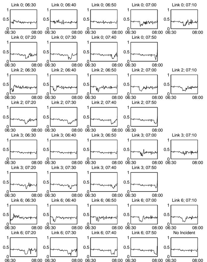
Fig. 6. Path 2 Flow Distribution of Routing Policy Model (X-Axis: Departure Time; Y-Axis: Path Share;  $p = 0.9$ ; Each subgraph represents a support point and the title indicates the incident location and starting time with the exception of the last one.)
