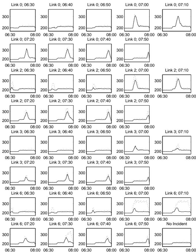
Fig. 5. OD Travel Time Distributions of Path Model (dotted) and Routing Policy Model (solid) (X-Axis: Departure Time; Y-Axis: OD Travel Time (sec);  $p = 0.9$ ; Each subgraph represents a support point and the title indicates the incident location and starting time with the exception of the last one.)
