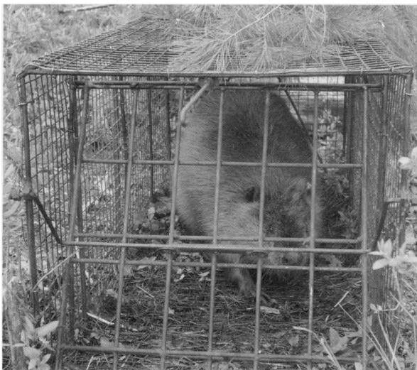
Figure 4. Drop-down bars, designed and installed by J. Benedetto of Animal Problem Control, Wakefield, Massachusetts, often were added to box traps to improve or replace the commercial locking mechanism.
