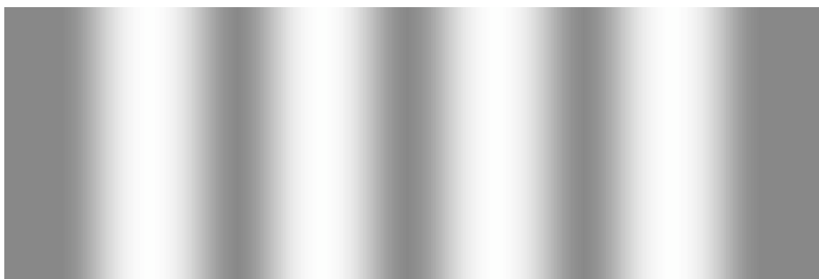
Figure 19. The pattern of light through two slits. At certain angles, the light from the two slits interferes and the light waves cancel each other. At the middle of the dark ridges are areas where no photons can hit the screen.
