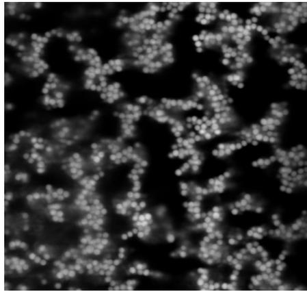
Figure 8. Slice of a gel of colloidal particles seen in confocal microscopy. The micrograph represents a  $44\ \mu\text{m} \times 40\ \mu\text{m}$  region at a depth of  $6\ \mu\text{m}$  into the sample away from the cover slip.
