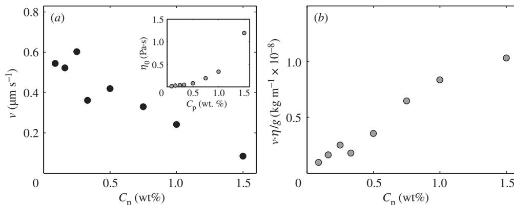
Figure 7. Sedimentation velocity,  $v$ , of the gel as a function of  $C_p$  for  $\phi = 0.11$ . (a)  $v$  calculated from the raw sedimentation-height data in the fastest part of the collapse where  $v$  is constant for each profile. Inset shows the zero shear viscosity of the suspending fluid plotted versus polymer concentration. (b)  $v$  normalized by the viscosity,  $\eta_0$ , versus  $C_p$ .
