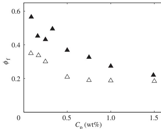
Figure 6. Comparison of final colloid volume fraction,  $\phi_f$ , of the collapsed state for starting volume fractions,  $\phi = 0.11$  (solid symbols) and  $\phi = 0.055$  (open symbols).  $\phi_f$  decreases as  $C_p$  is increased. The final state is more collapsed for starting volume fraction  $\phi_i = 0.11$  than for  $\phi_i = 0.055$ , with  $\phi_f$  approaching 0.20 at high polymer concentration in both cases.
