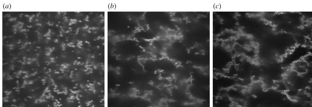
Figure 9. Structural evolution and coarsening during ageing of colloid–polymer mixtures. (a) 2 h, colloidal particles exist as monomers. (b) 1 day, colloidal network with only very few monomers remaining. (c) 4 days, the colloidal gel has aged, showing evidence of coarsening.
