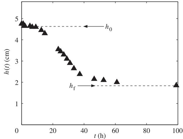
Figure 2. Schematic of the method used for normalization of sedimentation profiles prior to scaling: initial height of the colloid–polymer mixture,  $h_0$ , and the final height of the colloidal particles,  $h_f$ . In the fastest part of the sedimentation profile the slope is constant and yields the sedimentation velocity during the collapse.
