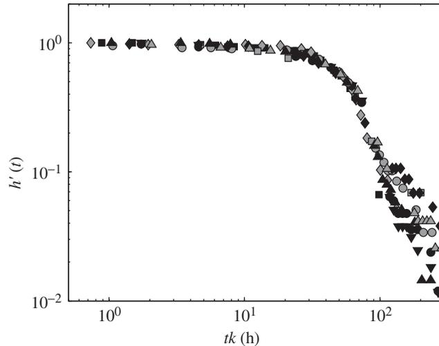
Figure 3. Master curve showing the normalized profiles as a function of scaled time for all data in figure 1, at  $\phi = 0.11$  and varying polymer concentration  $C_p$ . The scale factors yield the delay time  $\tau$  for the onset of the collapse for each polymer concentration.
