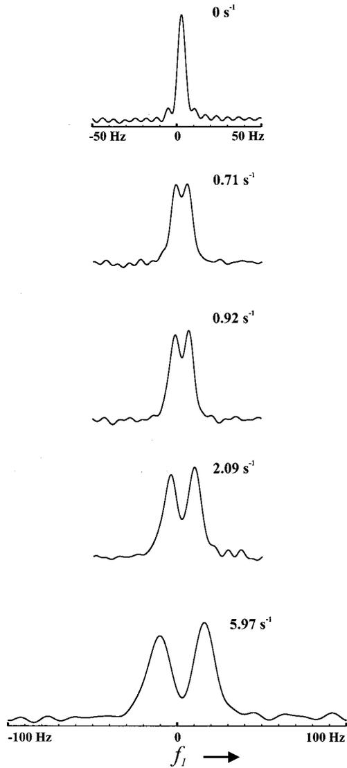
FIG. 9.  $^2\text{H}$  spectra obtained for a series of shear rates by Fourier transforming the signal evolution in the  $t_1$  domain. The spectra are plotted as signal amplitude versus frequency in hertz. The splitting arises from the electric quadrupole interaction with the  $\mathbf{B}_0$  field and is a measure of orientation in the polymer under deformation.
