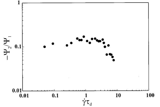
FIG. 12. Ratio of the second to the first normal stress difference, as given in Eq. (2) but calculated from the alignment tensor elements  $S_{XX}$ ,  $S_{YY}$ , and  $S_{ZZ}$ . Note the reduction about  $De \approx 3$ .
