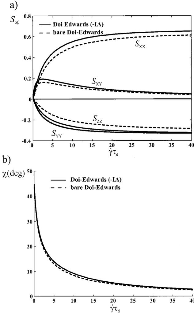
FIG. 3. (a) Elements of the alignment tensor  $S_{\alpha\beta}, \sigma_{\alpha\beta}$ , in terms of the reduced shear rate  $\dot{\gamma}\tau_d$ , calculated from the Doi-Edwards theory without the independent alignment approximation (—). As a comparison the bare the Doi-Edwards theory (---) is shown as well. (b) Extinction angle  $\chi$ , in terms of the reduced shear rate  $\dot{\gamma}\tau_d$ , as calculated from the Doi-Edwards theory without the independent alignment approximation (—).
