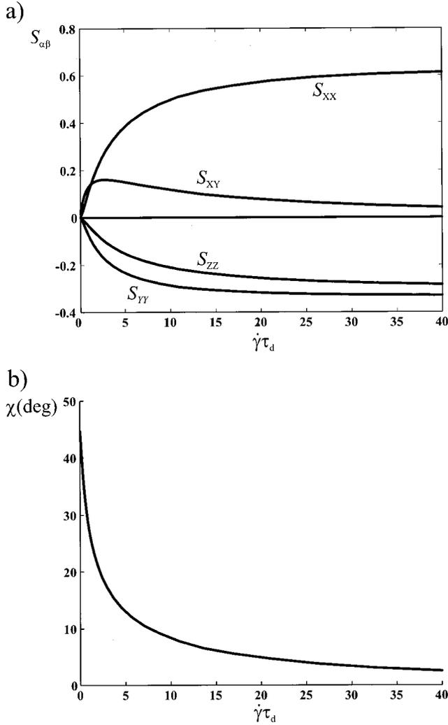
FIG. 2. (a) Elements of the alignment tensor  $S_{\alpha\beta}$ , in terms of the reduced shear rate  $\dot{\gamma}\tau_d$ , as calculated from the Doi-Edwards theory. (b) Extinction angle  $\chi$ , in terms of the reduced shear rate  $\dot{\gamma}\tau_d$ , as calculated from the Doi-Edwards theory.
