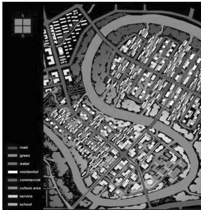
Figure 17.4. In the Taizhou “water town” alternative plan, the river is split and diverted through the city, managing the flood hazard and distributing the ecological functions provided by the river to residential neighborhoods (Turenscape, 2005)
