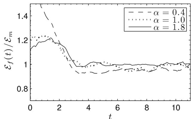
FIG. 1. Time evolution of the ratio of horizontal contribution to kinetic energy at the forcing plane to target energy for schema Rf.
