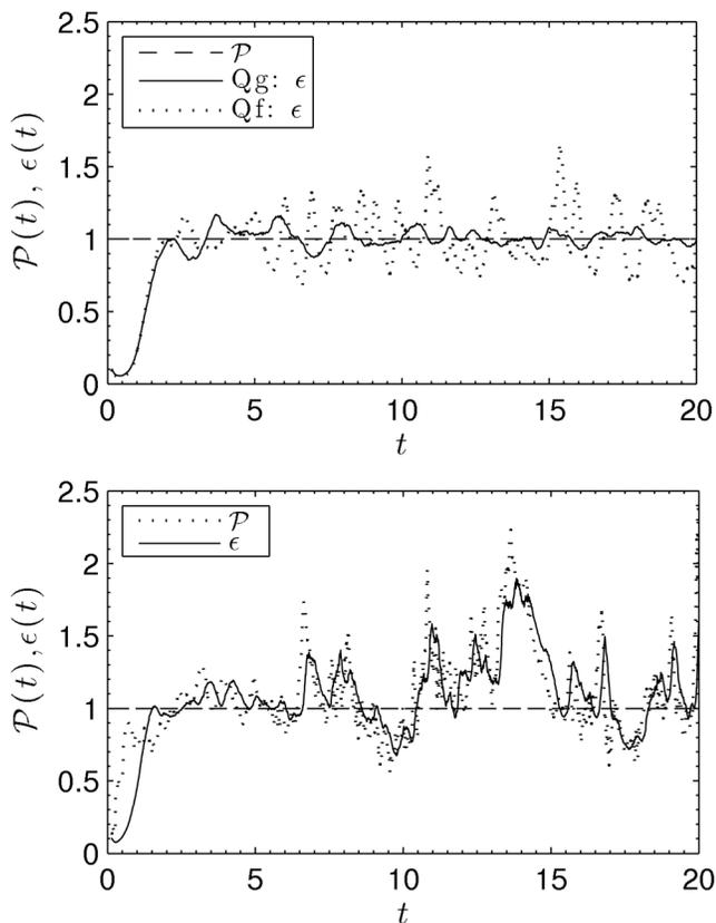
FIG. 4. Time evolution of spatially averaged energy dissipation rate,  $\epsilon(t)$  and forcing power,  $\mathcal{P}(t)$ . The top panel pertains to schemata Qf and Qg, while the bottom panel pertains to schema Rf.
