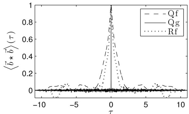
FIG. 3. The spatially averaged temporal autocorrelation of the force,  $\mathbf{b}$  for each forcing schema.
