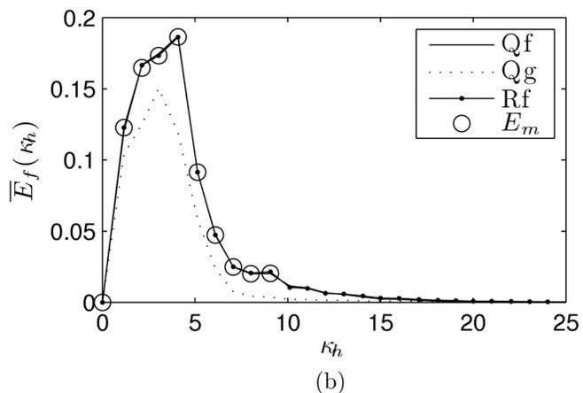
FIG. 2. (a) The agreement between forcing spectrum defined by Eq. (13) and actual injected forcing spectrum for the Qf and Qg schemata. (b) The agreement between model spectrum,  $E_m(\kappa_h)$  and  $\bar{E}_f(\kappa_h)$  for the Rf schema.
