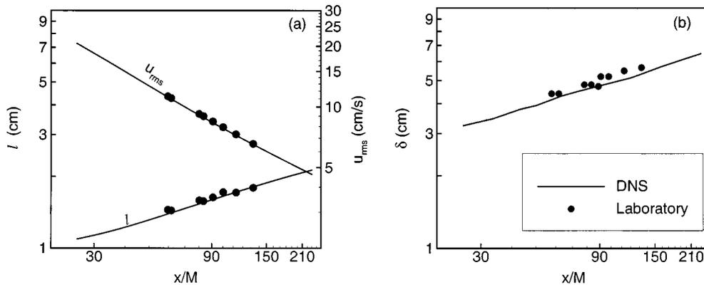
FIG. 2. Properties of the velocity and scalar fields. The symbols indicate laboratory data and the lines simulation results.
