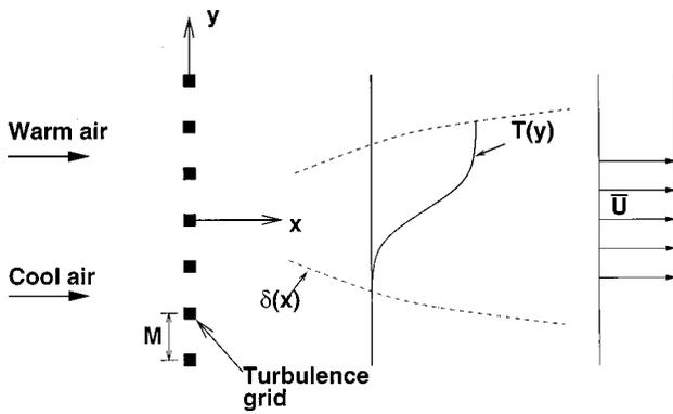
FIG. 1. Schematic of a thermal mixing layer.
